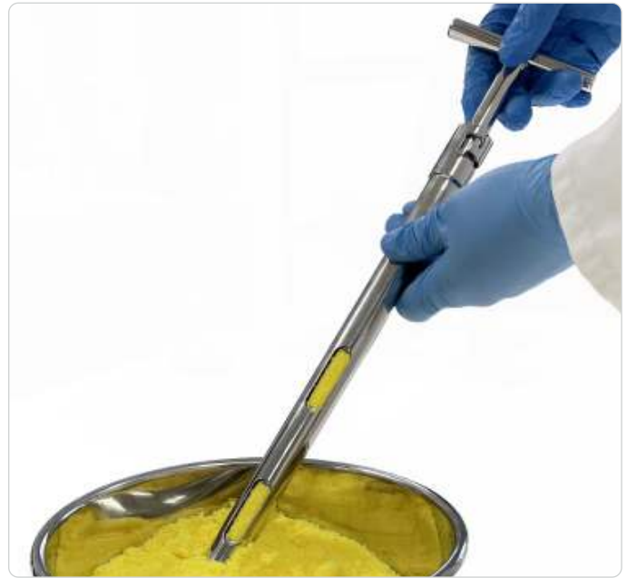
More than one sample can be taken from the same sampling point (see double or triple styles).
